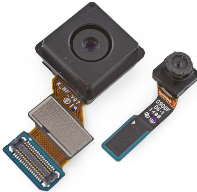
Figure 5: Samsung Galaxy S5 Camera Module (14)
